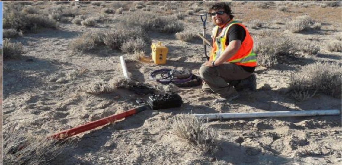
Various images above showing layout of field equipment including recording systems, cables, electrode and buried magnetometer sites.
