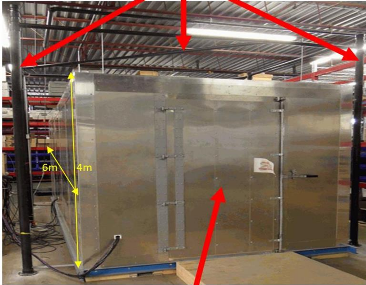
3-Layer Passive Magnetically Shielded Room
