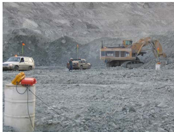
Figure 4. Distributed acquisition survey system collecting DCIP and MT data in active open pit mine. Receiver nodes shown with 50 m spacing in this application mapping side walls in kimberlite. Photo taken in Venetia Diamond Mine, South Africa.
