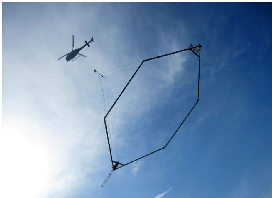
Figure 6. SkyTEM system acquiring TDEM data.
