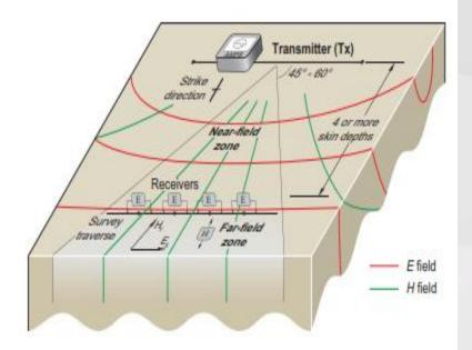
Figure A4.1 CSAMT survey arrangement. The transmitter dipole is oriented perpendicular to the geological strike (TM mode). Electric ( $E_X$ ) and magnetic ( $H_Y$ ) fields are measured in far-field zone.
