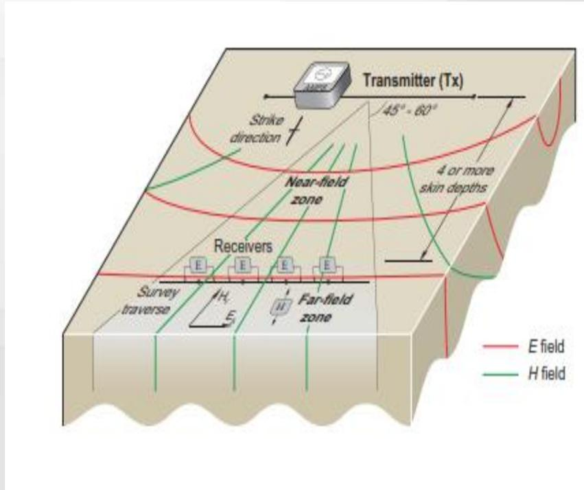
Figure A4.1 CSAMT survey arrangement. The transmitter dipole is oriented perpendicular to the geological strike (TM mode). Electric ( $E_x$ ) and magnetic ( $H_y$ ) fields are measured in far-field zone.
