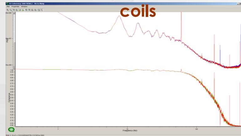
Power Spectrum (top) and coherency (bottom) of the coils from the TS shown above
