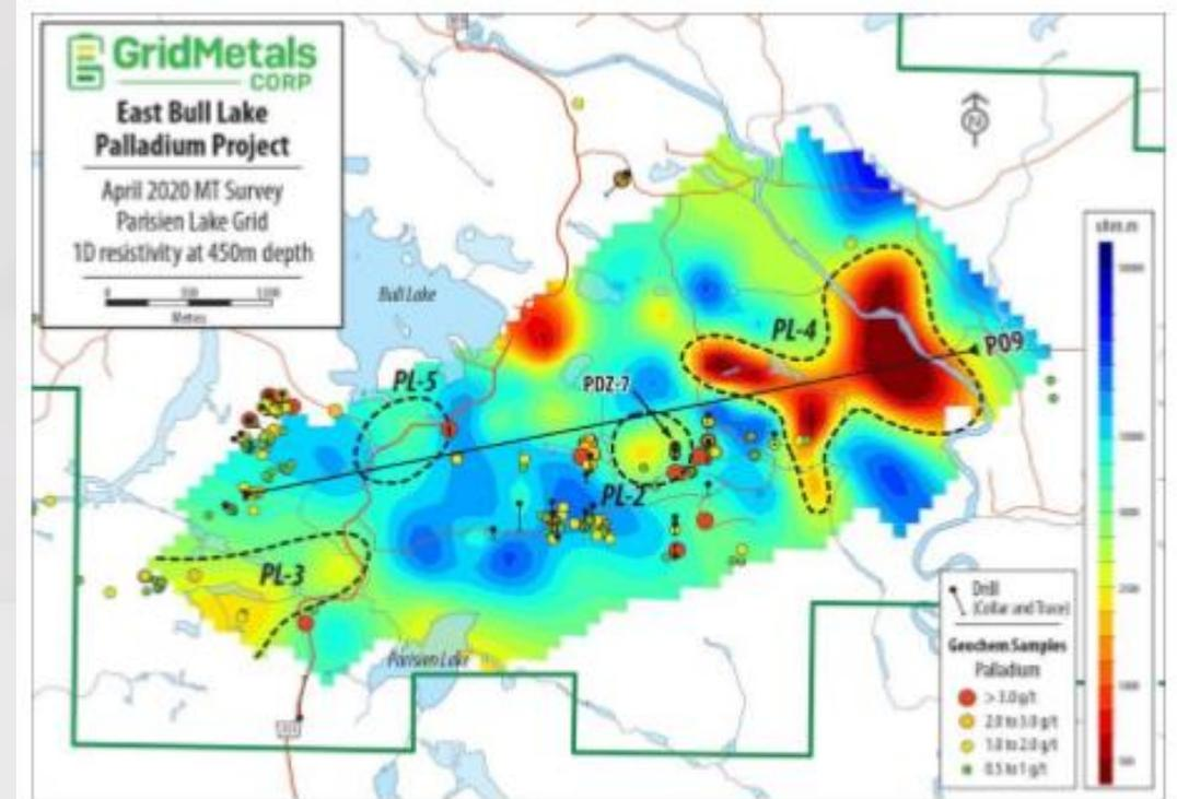
“The MT survey is an electromagnetic geophysical method with excellent depth penetration and a proven ability to detect, directly or indirectly, the type of palladium mineralization (high palladium tenor disseminated sulfide) that is found at EBL. Initial results from the completed portions of the survey have delineated several high priority geophysical targets proximal to known palladium rich mineralization. “
