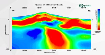
Portable, excellent tool for remote imaging, example geothermal exploration (4km depth)
