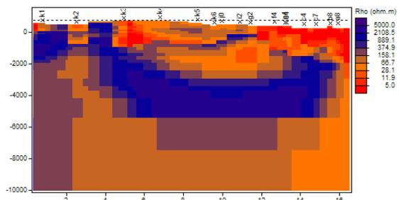
Figure 6. TE+TM-mode 2D inversion model using an a priori model based on the geological section in Fig.3 along profile AA' (SW on the left, NE on the right).
