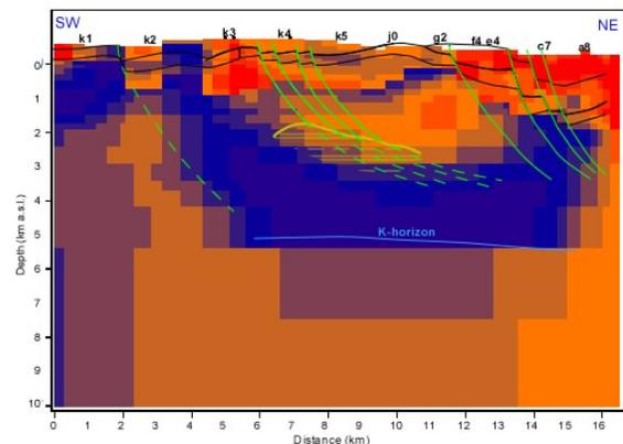
Figure 7. Resistivity cross-section overlapped by the geological model.
