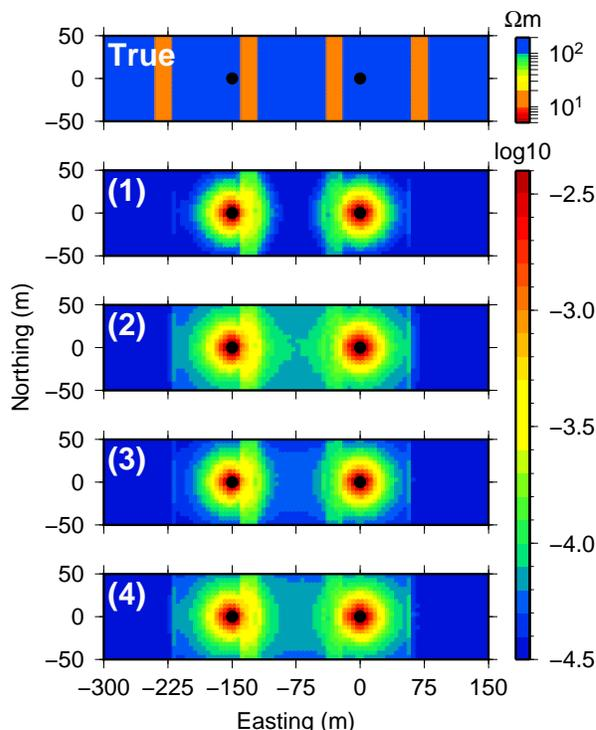
Figure 4: Plan-view sections of the sensitivity at an elevation of 215 m calculated using the probing method with 5 iterations for each of the four surveys. In each case, there is higher sensitivity to the left chamber than the right. Even though there are chambers on the other sides of the two vertical wells, none of the surveys are sensitive to those regions. The top panel shows a plan-view section through the true model, shown in Figure 1.
