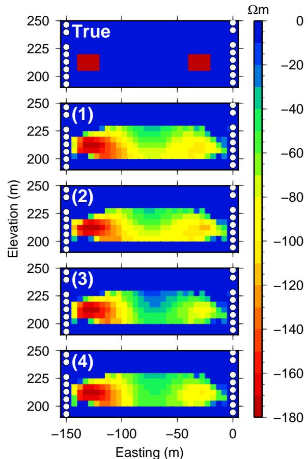
Figure 5: Each panel shows the recovered models at a northing of 0 m for the four different surveys. Only the reservoir portion is shown as only these cells were allowed to change resistivity in the inversion. Color scale indicates the change in  $\Omega\text{m}$  from the initial model.
