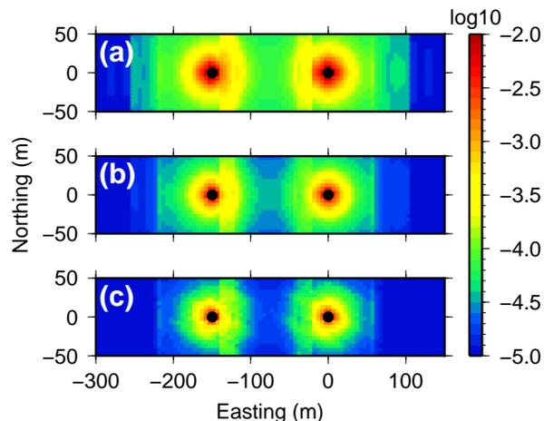
Figure 3: Plan-view section of the sensitivity at an elevation of 215 m calculated using the probing method with (a) 1, (b) 5, and (c) 15 iterations.
