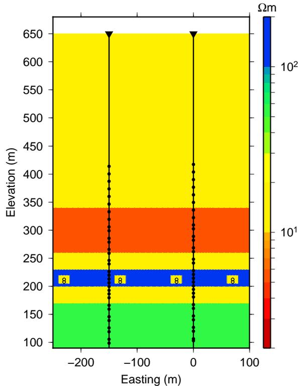
Figure 1: The geology at Leismer is modeled as a 1D layered earth with 4 SAGD chambers added. The figure shows a slice through the 3D model at a northing of 0 m. Two observation wells are located at an easting of 0 m and -150 m and contain electrodes, indicated as black dots. The horizontal well pairs, indicated using black circles, are at easting values of -230 m, -130 m, -30 m, and 70 m.
