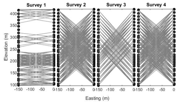
Figure 2: Four DC resistivity surveys collected at the Leismer Demonstration Area to monitor steam chamber growth. Black dots indicate electrode locations. Grey lines connect transmitter electrodes. Surveys 1, 3, and 4 also have along-well transmitters (not shown).
